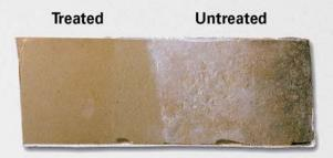
Drywall treated with Bora-Care with Mold-Care and placed in an incubator for 90 days.
