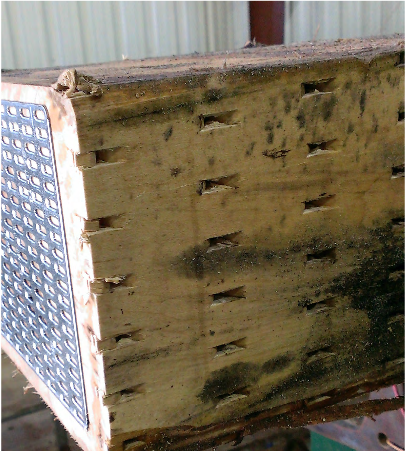
FIGURE 12. The incising of this tie will help penetration during pressure treatment. The end plate will reduce the severity of end splits.
