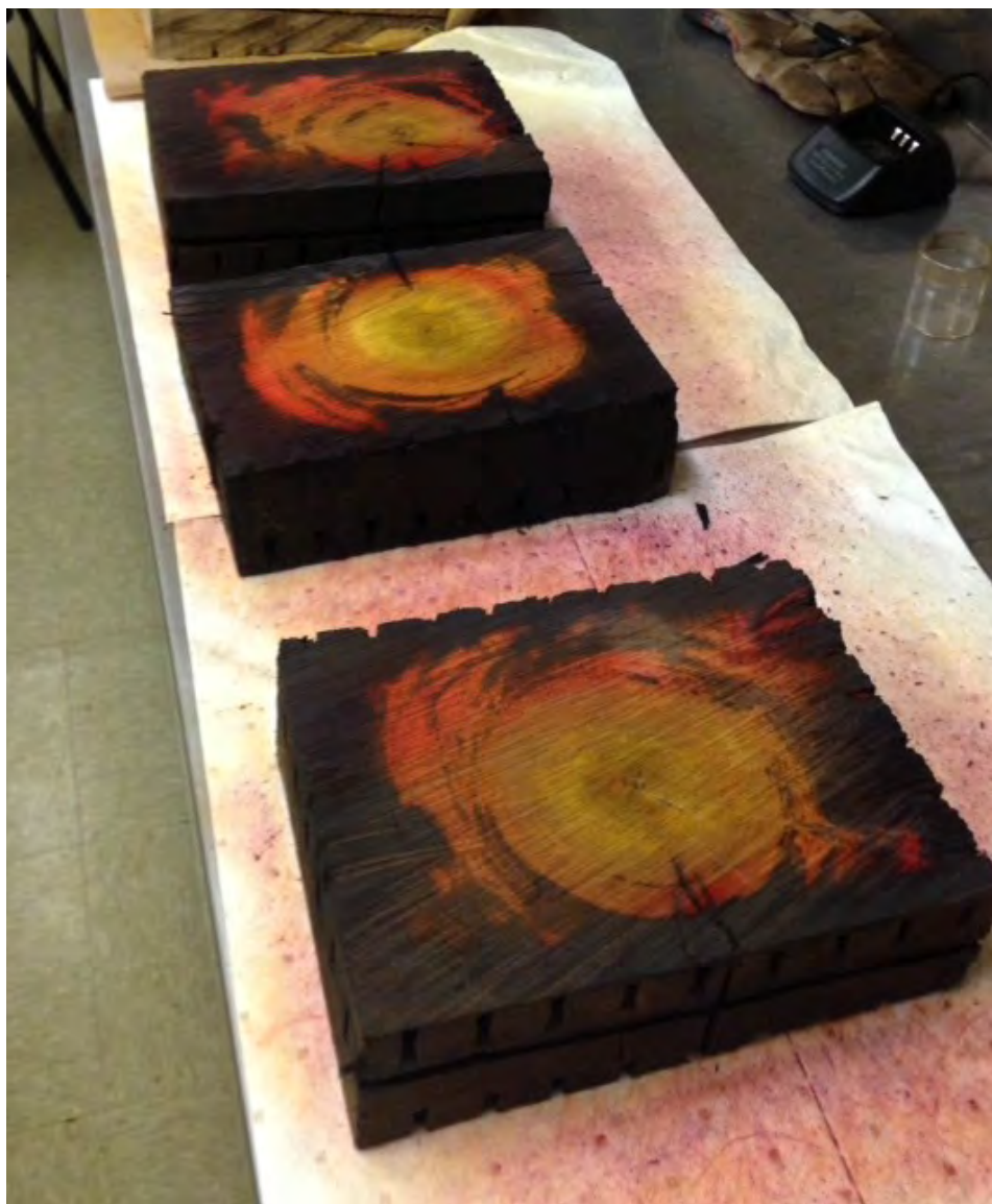
FIGURE 14. A dual-treated (two step) tie. The inner portion not penetrated by the creosote treatment is protected by the borate (curcumin sprayed to show boron as red).
