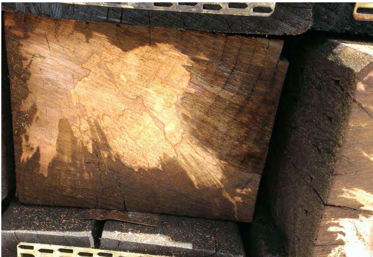
FIGURE 9. Stack burn weakens wood and can also interfere with treatment. Fungal activity can increase moisture content locally. Creosote failed to penetrate the areas where the fungus was established in this tie. The untreated areas are prone to decay in service.
