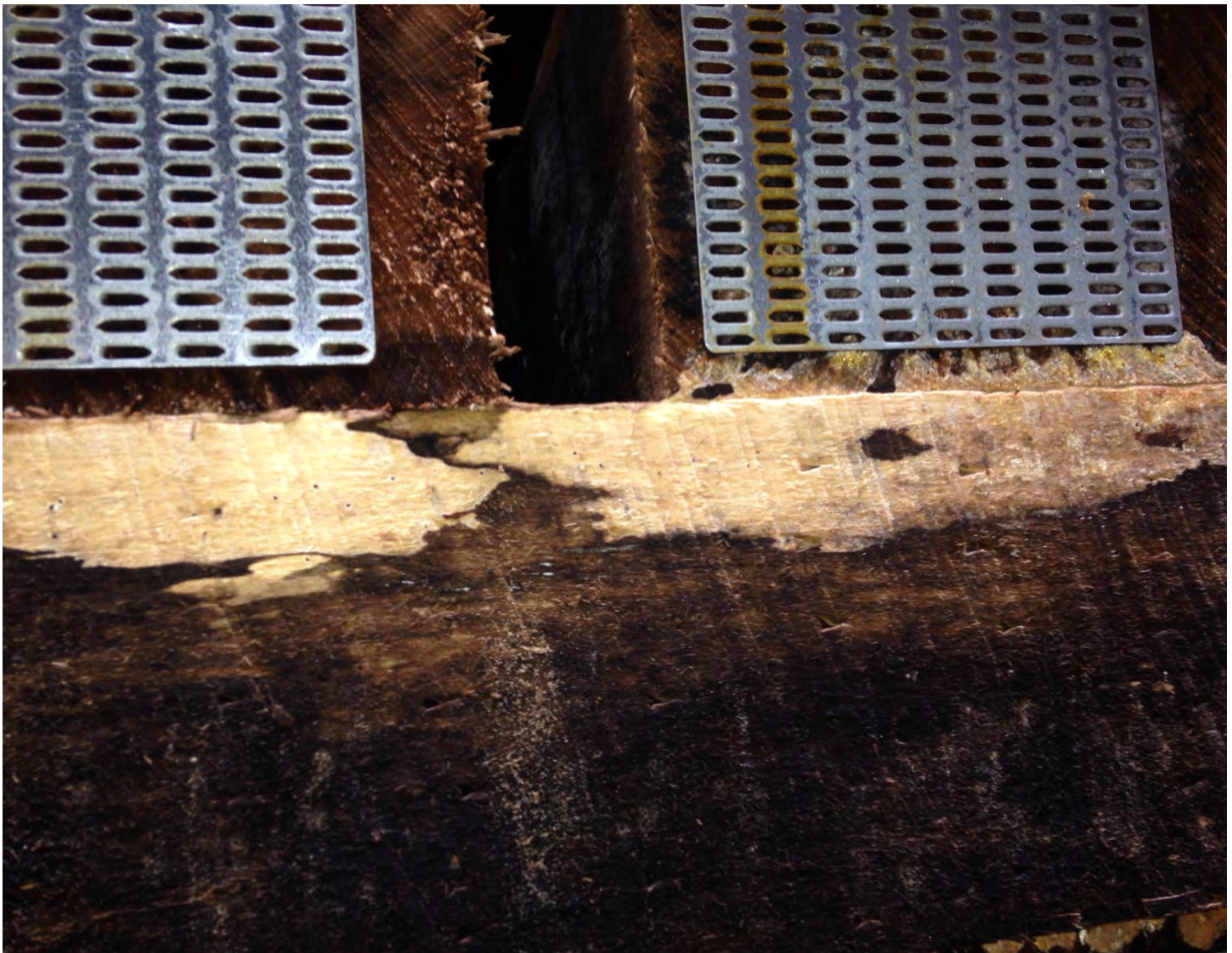
FIGURE 7. The white areas are rotten. This “stack burn” is occurring at the touch points between ties, where drying is retarded.
