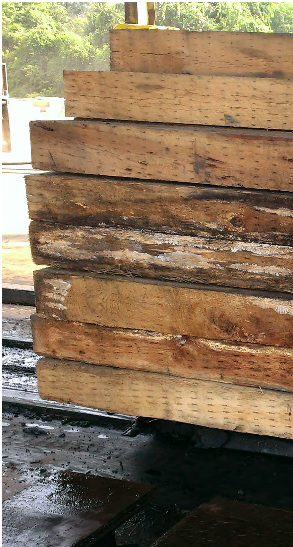
FIGURE 8. Stack burned (partially rotten) ties going into the treatment cylinder. These ties have lost some of their potential for excellent service and this loss cannot be recovered.
