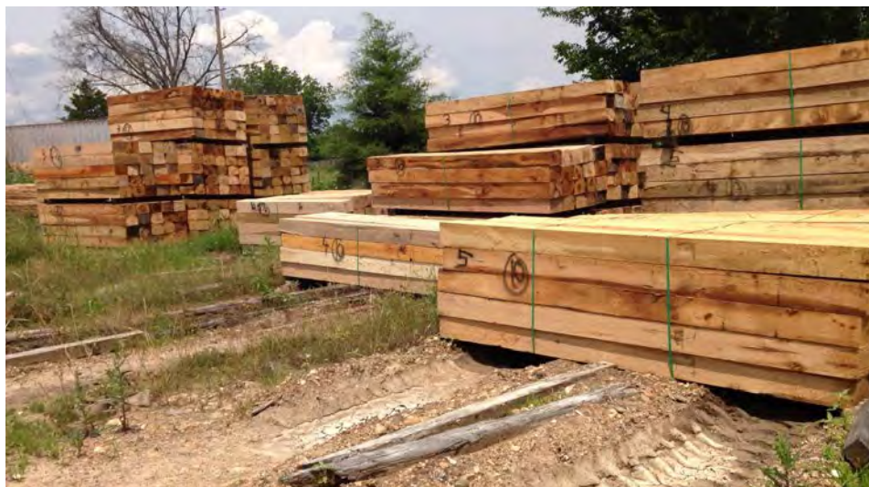
FIGURE 3. Dead stacking nonseasoned ties prevents drying and will quickly lead to decay and/or insect damage. Soil contact during storage or drying is also to be avoided.
