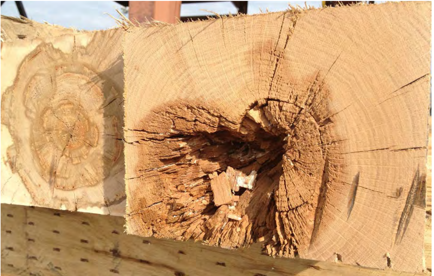
FIGURE 1. The rot in this freshly cut tie occurred in the living tree. It should be culled.
