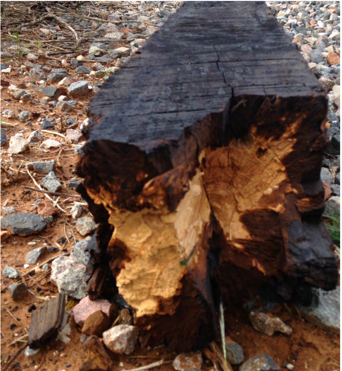
FIGURE 11. Stack burn ruined this tie before it was treated. The blunt (“brash”) break of the wood in this tie is typical of the effects of fungal decay. Decay also increases permeability. The creosote treatment here shows excellent penetration. Unfortunately, the creosote preservative was applied after the damage was already done.
