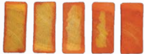
Under ideal conditions, Bora-Care penetrates wood over a 4-6 week period and remains for the life of the wood.
