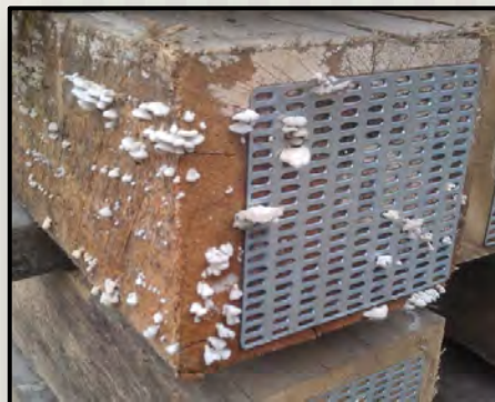
With 2-Step Dual Treatment, internal decay during air drying is virtually eliminated.
