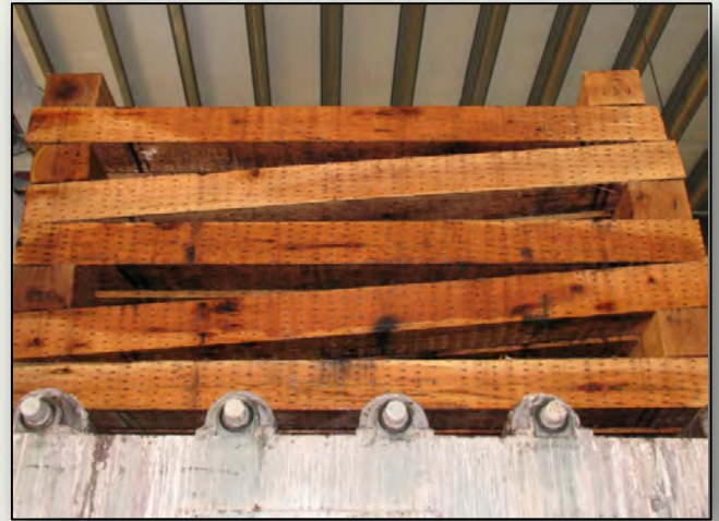
German stacked ties are dip treated in Cellutreat Liquid Borate DOT
