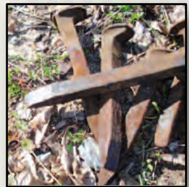
Clean, shiny spikes after 23 years of service illustrate boron corrosion-inhibiting properties.
