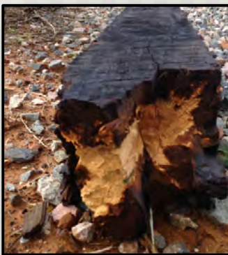
Brash failure during installation. Good preservative penetration, but internal decay caused failure.
