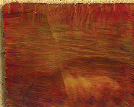
Gum tie dip treated with Cellutreat and then pressure treated with QNAP.*
