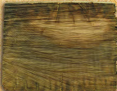
Gum tie air-seasoned and then pressure treated with QNAP copper naphthenate.
