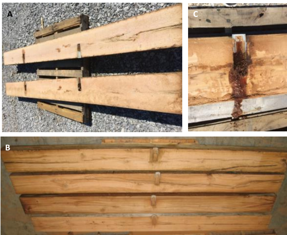
Figure 2: Freshly cut surfaces of bridge ties after 14 (A) and 40 (B) weeks of the treatment. Some residual liquid borate was found inside of the hole (C) while no liquid borate was found in the all 40-week-old ties (B).
