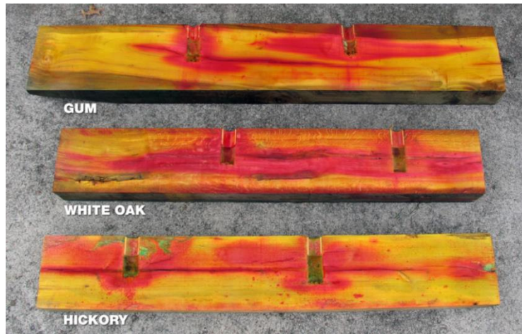
Figure 3: Presence of DOT (red) in freshly cut bridge ties tested 3 weeks after Boulton conditioning and treatment in copper naphthenate.
