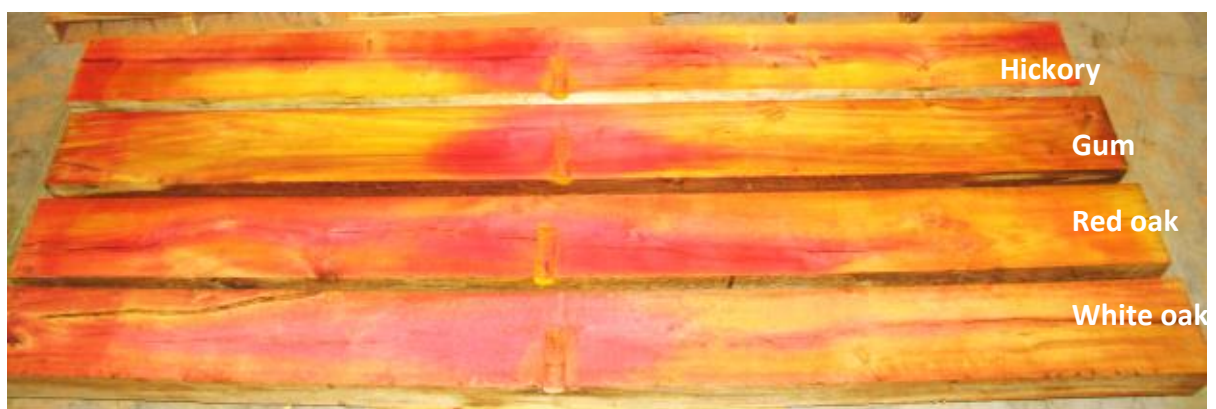
Figure 5: Presence of DOT (red) in freshly cut bridge ties tested 40 weeks after Boulton conditioning and treatment in copper naphthenate.
