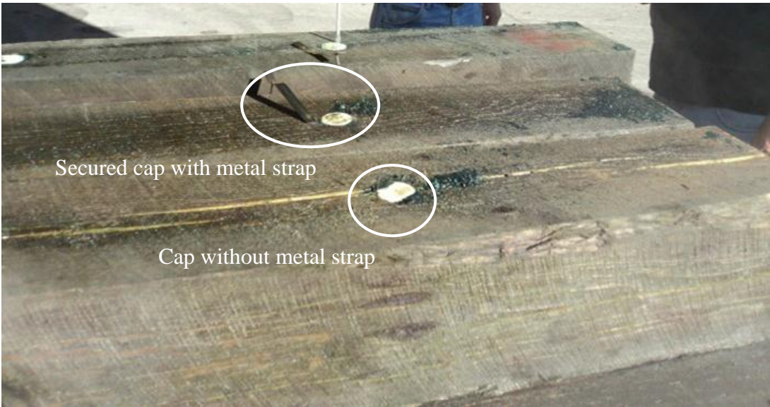
Figure 5. Cap on the third timber was not secured and the cap stayed in place after pressure treatment with QNAP.
