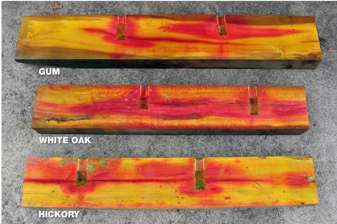
Figure 7. Diffusion of DOT in freshly cut bridge tie. Significant longitudinal diffusion was observed.
