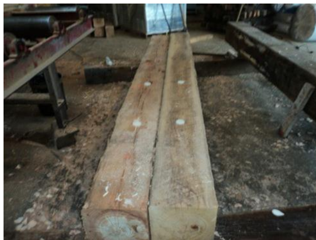
Figure 2. Capped 2" (2.5cm) holes
