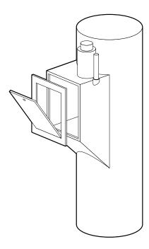
Figure 1. This round chute shows a typical square door system, which has many areas where food can collect and provide more than adequate food sources to sustain cockroaches and other insect pests. The round design works better than old Square chutes, but is still not totally self-cleaning.
