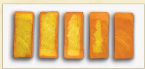
An added colorant demonstrates Bora-Care's penetration into wood.
