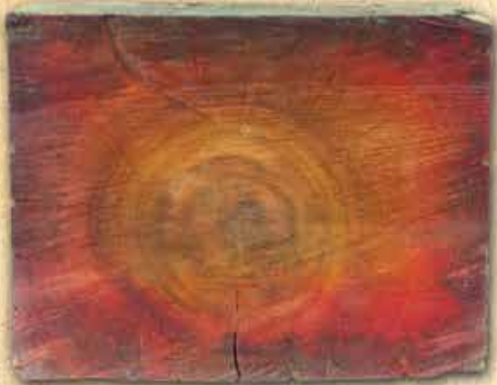
Diffusion of Cellutreat into hardwood (gum) shown by red curcumin indicator.
