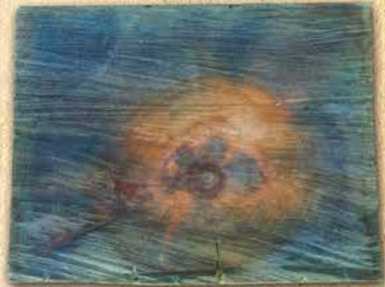
QNAP penetration into hardwood (gum) shown by blue Chrome Azurol S indicator.
