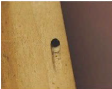
Powderpost beetle exit hole.
