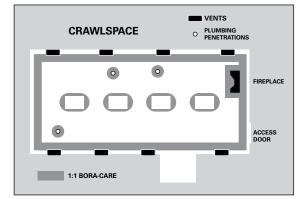
component that extends directly from the soil towood. This includes the subfloor, floor joists and any other wood in contact with the support pier. Normal crawlspace piers should be measured at eight linear feet of treatment area per pier. To obtain the amount of Bora-Care solution needed, multiply the number of piers by eight and divide by 100 (the number of linear feet covered by 1 gallon of Bora-Care solution).
