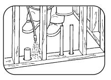
Interior and exterior walls, the slab, plumbing penetrations and bath traps are treated on slab structures.
