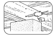
If desired, JECTA is injected into tripled or quadrupled support members to insure coverage.
