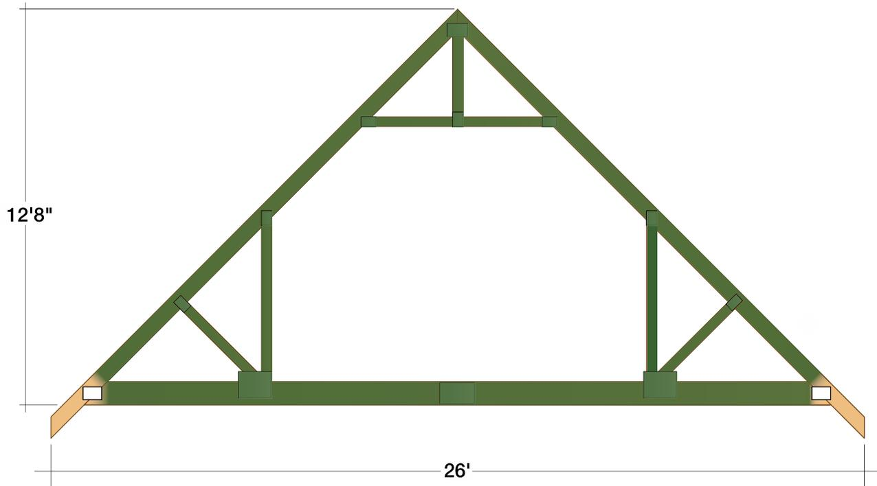
**Figure 5:** Attic truss
